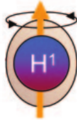
Figure 1: We can visualise the Hydrogen atom as a charged sphere spinning, that give rise to a small magnetic moment (in yellow) [9]
